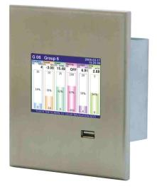
Panel or in-wall mount MultiCon CMC-99SL is featured by a shallow casing - only 50 mm! All connectors are introduced on side walls of the device as in a typical panel computer. As the number of measurement inputs and outputs is limited, this design in intended mainly for systems with a small number of signals or systems which include other measurement systems with Modbus RTU interface. An Ethernet interface is also available to upgrade every MultiCon control's application easily.
